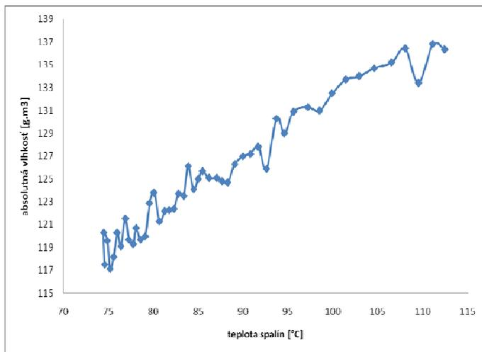
Fig.2 Dependence of absolute combustion product moisture on combustion product temperature
