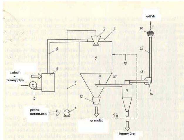
Fig 1 - Sprinkle kiln [1]
