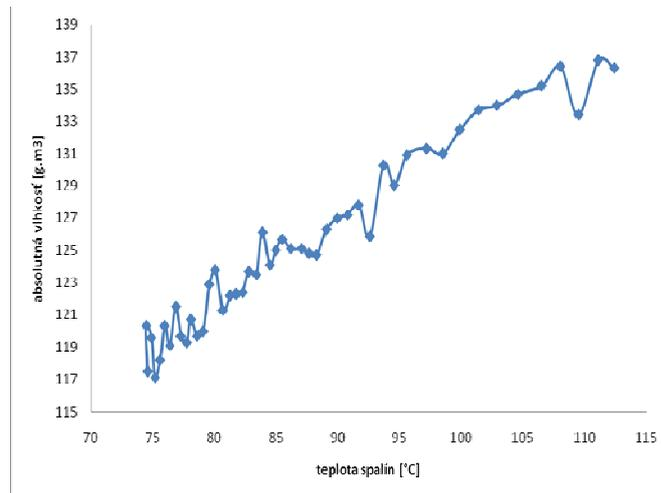
Fig.3 Absolute combustion moisture dependence on the combustion temperature
