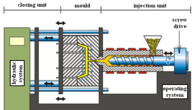
Fig. 1. Basic parts of injection moulding machine
