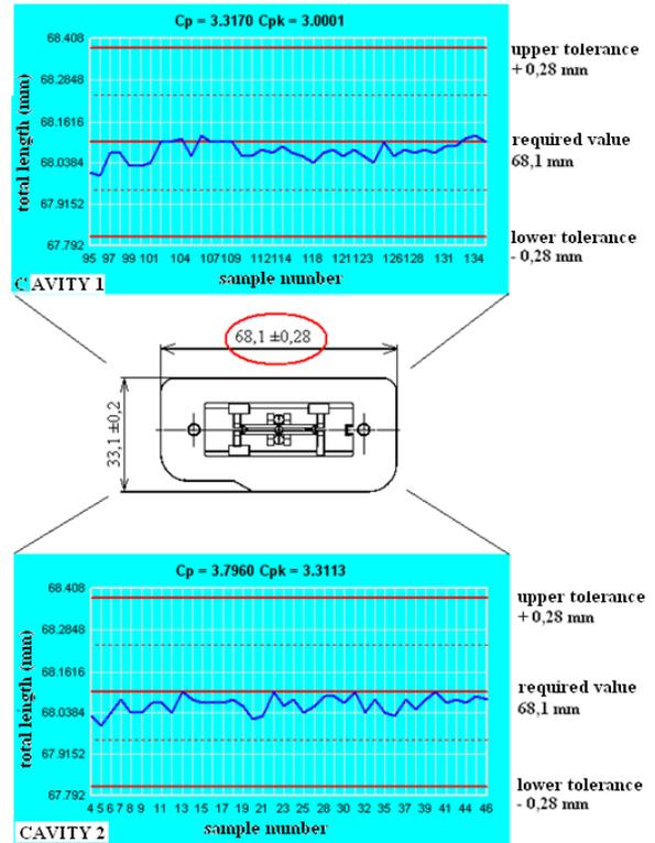
Fig. 11. Measuring of total length  $l_2$
