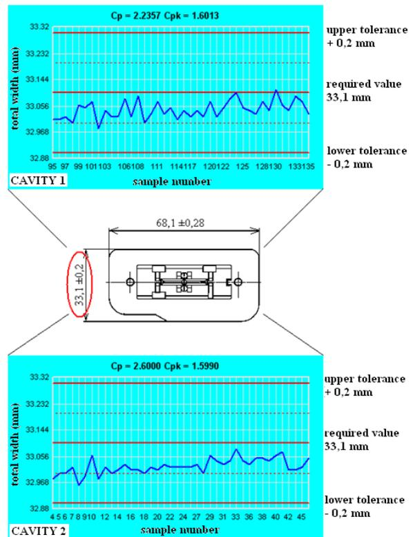
Fig. 12. Measuring of total width  $s_2$
