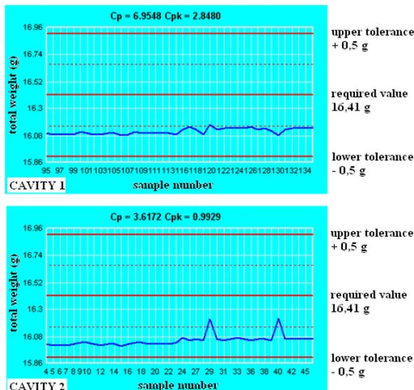
Fig. 13. Measuring of total weight  $m_2$
