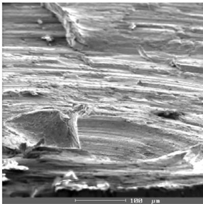
Fig. 1 Plastic deformation alongside machined surface of stainless steel by drilling, REM
