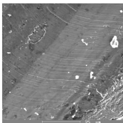
Fig. 4 Plastic deformation in cutting zone, on the machined surface, steel 1.4301
