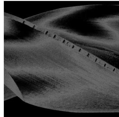
Fig. 2 Thermal analysis on the minor cutting edge by screw drill (black place – 620 °C)
