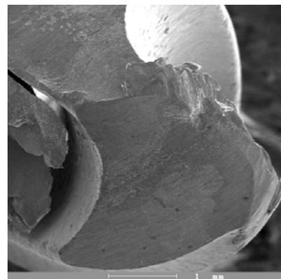
Fig. 3 The base tool wear mechanism - plastic deformation of major cutting edge
