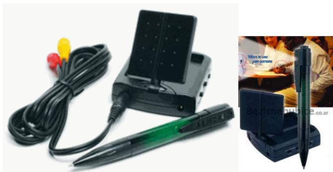
Fig. 3. Micro camera in a pen
