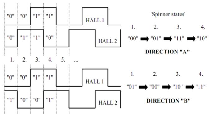
Fig. 6. Hall sensors signal demodulation [7]
