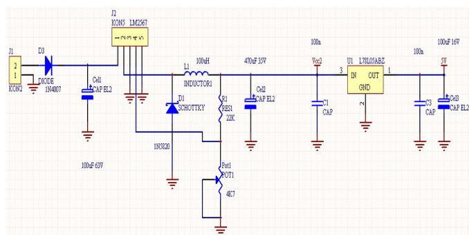
Fig. 7. Scheme of voltage regulator circuit on digital board
