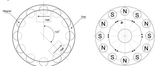
Fig. 4. Position of two Hall sensors relative to magnets and permanent magnets placement and their magnetic field B
