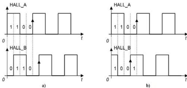
Fig. 5. Digital outputs of the sensors in case of a) counterclockwise rotation and b) clockwise rotation
