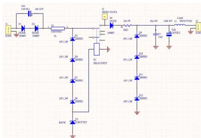
Fig. 8. Scheme of voltage regulator board
