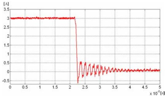
Fig. 5. Turn-off current of the proposed com-bined MOSFET-IGBT leg (lack of tailing current)
