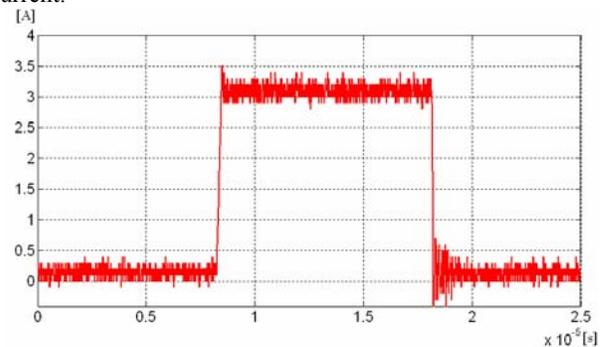
Fig. 3. Turn-on current of the proposed combined MOSFET-IGBT leg (less turn ON switching losses)
