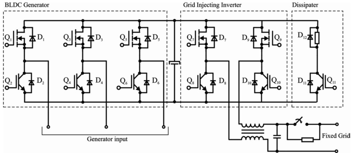
Fig. 9. IGBT – MOSFET topology for Combined Heat and Power system
