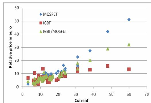
Fig. 8. MOSFET and IGBT availability in relation to power ratings.
