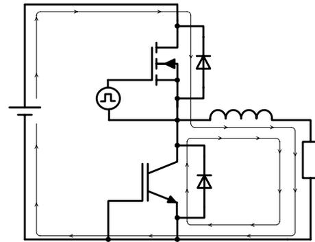
Fig. 1. Suggested MOSFET and IGBT combined Leg
