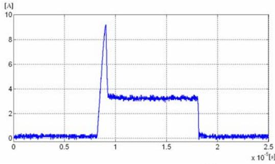
Fig. 4. Turn-on current trough a pure MOSFET leg.
