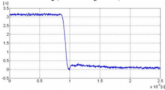
Fig. 6. Turn-off current trough a pure IGBT leg.
