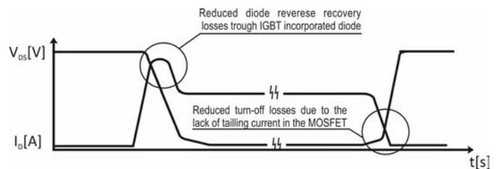
Fig. 2. Switching loss reduction.
