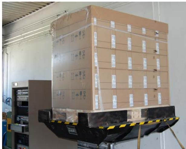
Fig.2 Vibration test on transport packaging
