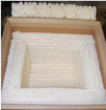
Fig. 6. Thermobox with biodegradable cushion (source: own photo 2009)
