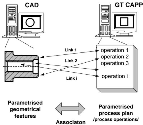
Fig.7. Principle of parametrisation and association in GT CAPP
