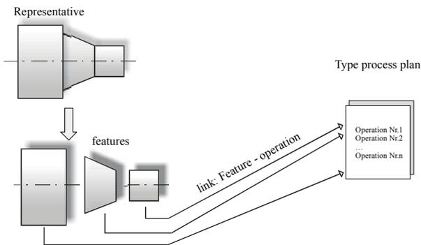
Fig.6. Association - links between parametrised design features and process operations
