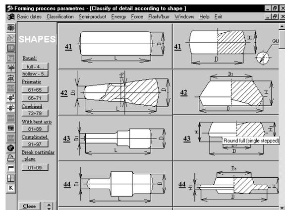
Fig.2. Developed visual classification according the geometry
