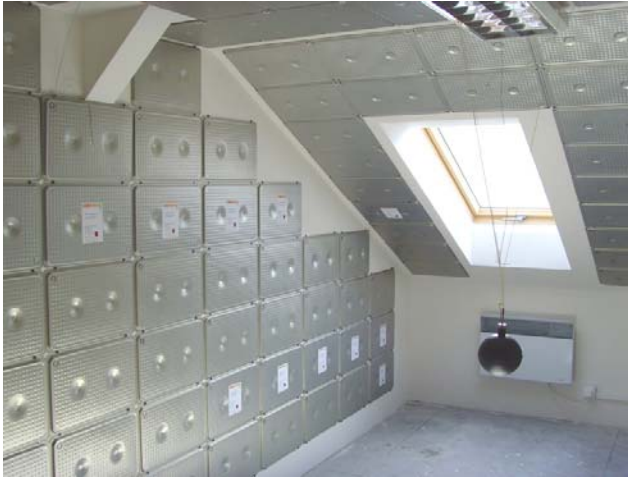
Pict. 2. Experimental room with panels of PCM
