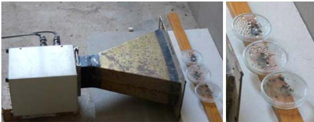
Fig. 3 Application of EMW radiation on the mould samples
