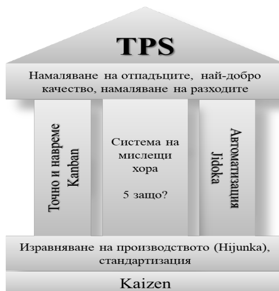
Fig. 1. Elements of TPS (source TOYOTA PRODUCTION SYSTEM. A system or a philosophy? https://www.researchgate.net/publication/312213247_TOYOTA_PRODUCTION_SYSTEM_A_system_or_a_philosophy )
